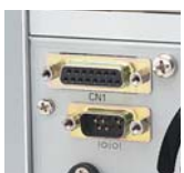
Upper: D-SUB connector Under: RS-232C
